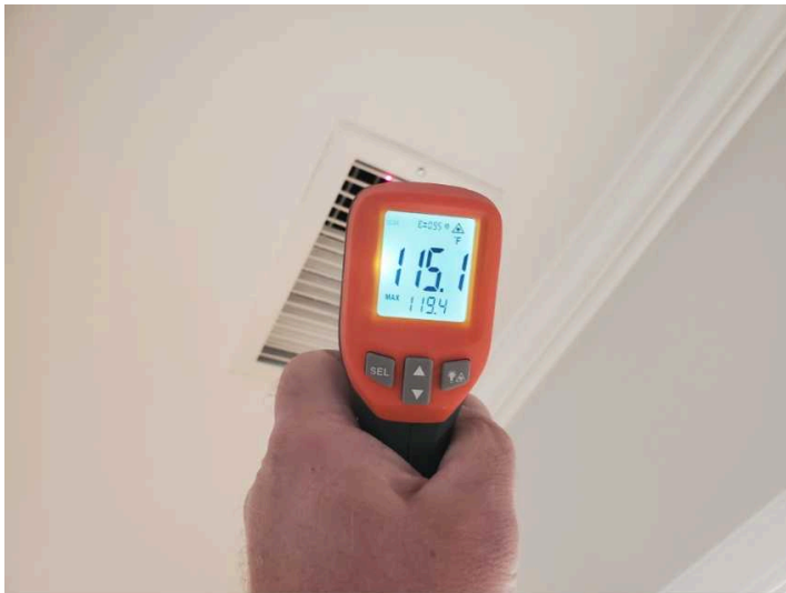
Heated temperature at register in front room
