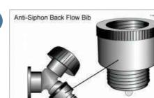
e anti-siphon bib device prevents contaminated water from backing up into potable water supply via a siphon effect. The anti-siphon device screws to the threaded hose bib and is secured by using a set screw.
